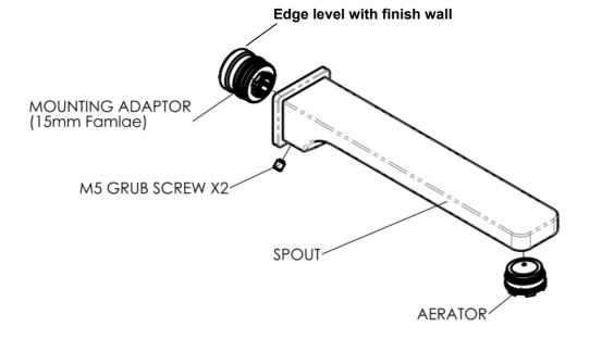
Install a brass 15mm male wingback elbow (not supplied).1. Note: Mounting adaptor requires MAX 15mm thread from finished wall.
