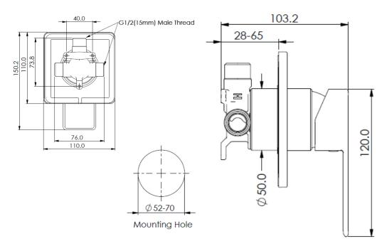
CHECK: Jet in body MUST fit inside the swivel nut connector.
