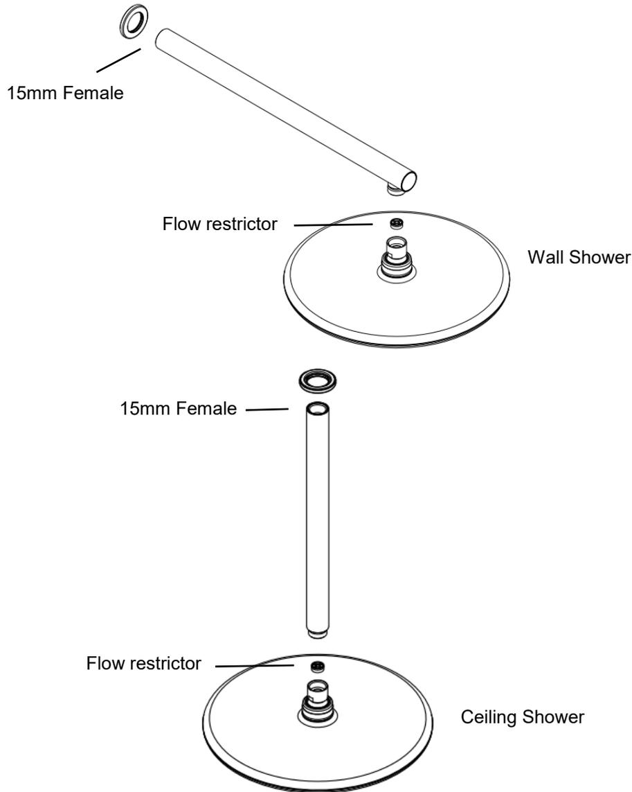
1. Position trim ring over the wall arm and remove the protective tape from seal on trim ring.
