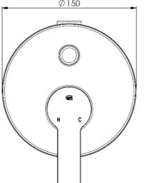
Note: The Mixer can be mounted 48mm to 73mm behind finished wall surface. Locate the correct position of the mixer by ensuring the "Hot" inlet, enters from the left. The top outlet is for the shower the bottom outlet for the bath. Ensure the diverter button is above the handle when the valve is fitted.
