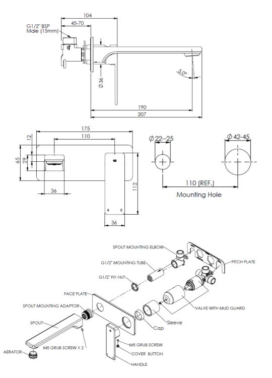
NOTE: Spout can be installed on the left or right side of the mixer valve.
