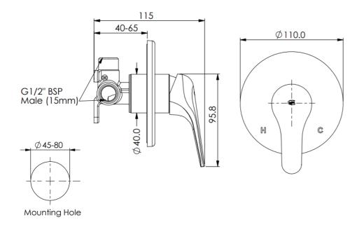
Note: The Mixer can be mounted 40-65mm behind finished wall surface.
